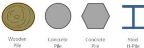
Concrete piles are pre cast, that is, made at ground level, and then driven into the ground by hammering - more on that later. Steel H-piles can also be driven into the ground. These can take very heavy loads, and save time during construction, as the pile casting process is eliminated. No protective coating is given to the steel, as during driving, this would be scraped away by the soil. In areas with corrosive soil, concrete piles should be used.
